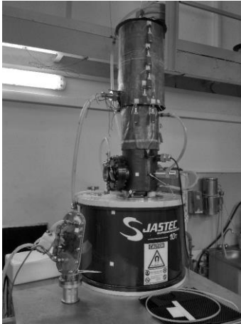
Fig. 1. Photo of the gyrotron in the cryomagnet.
