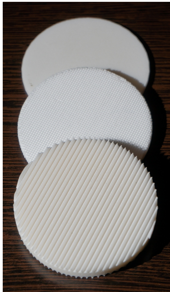
Fig. 3. Printed discs for antireflection grating tests: top – no gratings, middle – pyramidal gratings, bottom – one-dimensional gratings.
