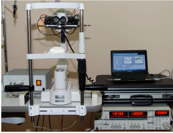
Fig. 1. THz reflectometer setup embedded into ophthalmic apparatus
