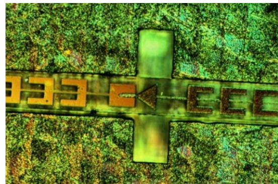
Fig. 2. Photo of the integrated mixing structure after installation in the mixer block
