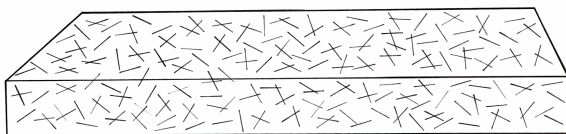
Fig. 1. THz radiation sources in the form of a matrix transparent in THz wavelength range with embedded GNBs
